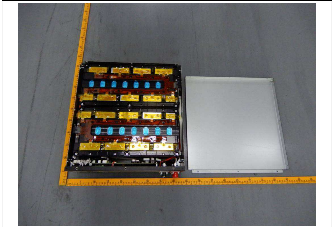
Internal view-1 of battery
