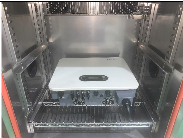
No.5 Low temperature, dry heat, temperature change and cyclic damp heat test.
