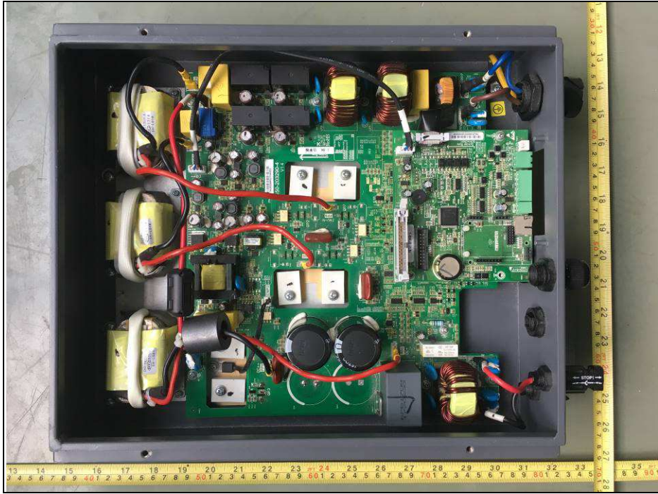
Internal view of SOFAR 1100TL
