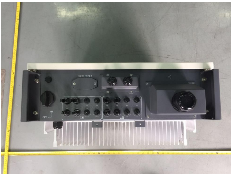
Photo29 ( Terminal interface ) SOFAR 20000TL
