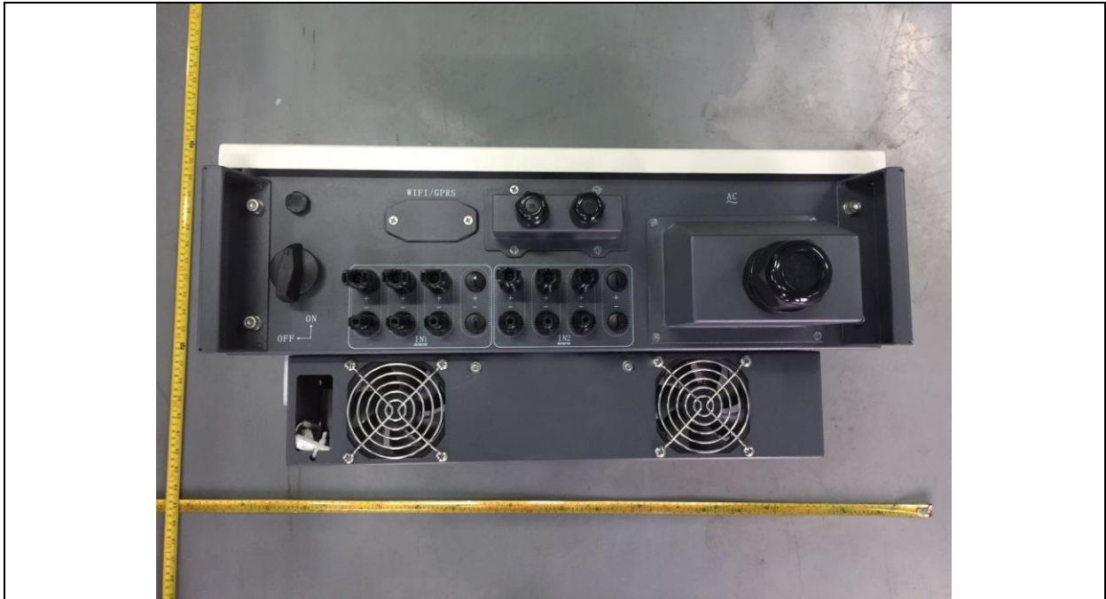
Photo30 ( Terminal interface ) SOFAR 25000TL
